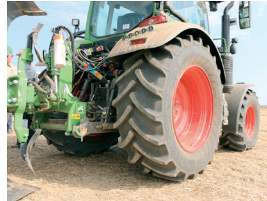
Mitas SST tires reduce the so-called booming noise.
